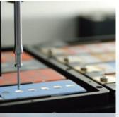
IFA tests on slides are performed as screening and/or titration, with a serial dilution capability.
